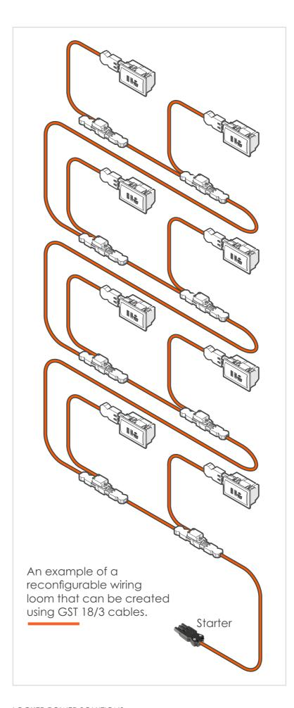
Click-and-connect wiring makes installing OE units into lockers quick and easy. Simply snap the unit into a suitable cut-out, then create a reconfigurable wiring loom from GST 18/3 power cables.
