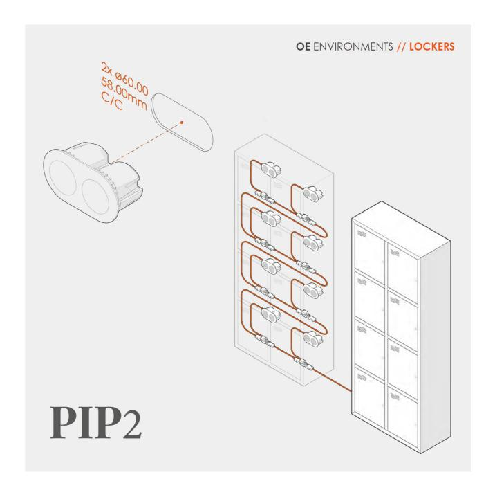
PIP2 can be configured with two OE Elsafe mains AC sockets or two TUF-R USB charging modules, or one of each.
